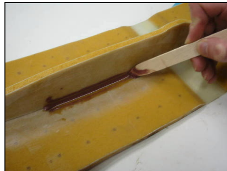
Figure 30: Placing the fillet
