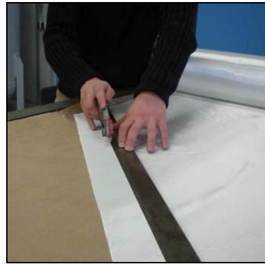
Figure 12: Cutting with a rotary cutter
