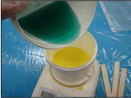
Figure 27: Mixing a fillet
